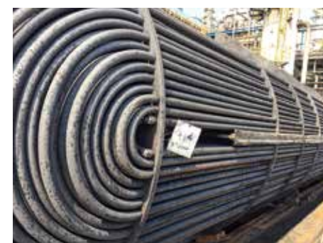
FIG. 1. The inspection revealed no visible signs of corrosion or fouling in the reactor section, coalescers, fractionation system or the reboiler bundle for the DIB column, shown here.
