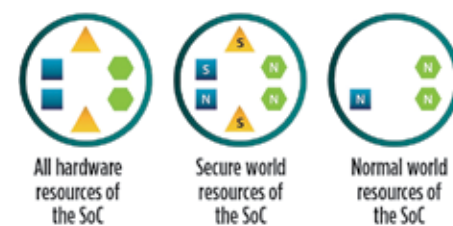
FIG. 1. TrustZone® technology allows developers to designate functions within a SoC as “secure world” or “normal world.”
