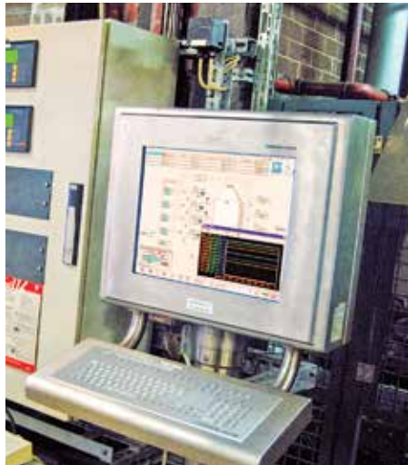
FIG. 1. While the user operates the dedicated workstation as usual, the host server generates the user interface, compresses it and sends it through an Ethernet-based remote protocol to the thin client.
